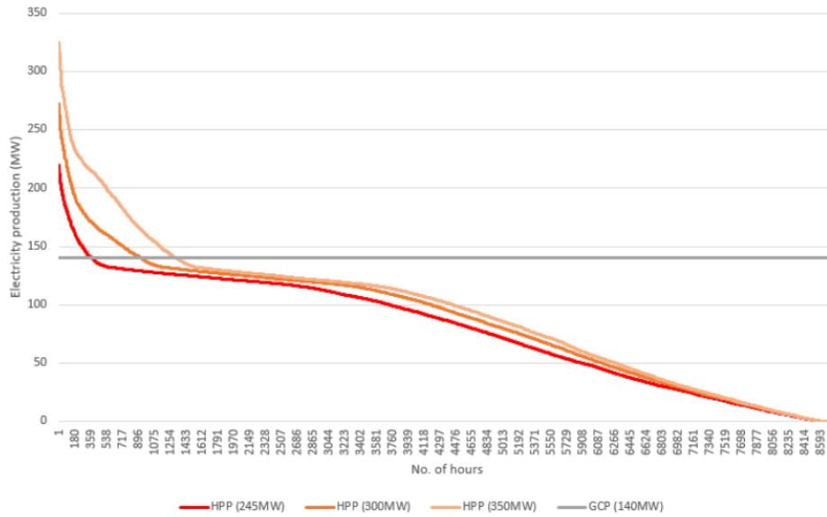
Figure 8.2: Duration curve of electricity production from different sizes of the hybrid power plant.
